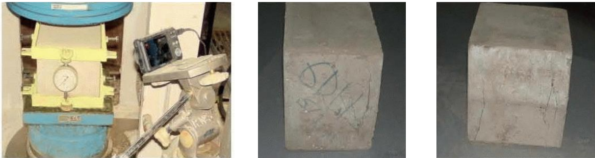
Figure 4. Appearance of failure modes of strong mortar cubes after the loading.
