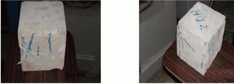
Figure 3. Appearance cracking of weak mortar cubes after loading (Failure modes of mortar cubes).
