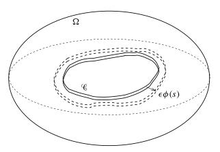
Figure 1. Slight in-plane perturbation of a plane crack in an arbitrary body.
