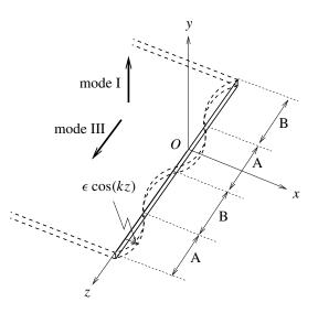
Figure 5. In-plane sinusoidal perturbation of a semi-infinite crack loaded in mode I+III.
