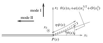
**Figure 4.** Geometric hypotheses and notations for Cotterell and Rice's directional stability analysis of a propagating crack.
