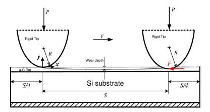
**Figure 2.** Schematic of peridynamics wear model of a sharp conospherical diamond (rigid) tip under a normal load P sliding at a constant velocity V and plowing through a thin a-C film, which is firmly attached to a thick Si substrate. The tip slides against the film surface from left (x/S=0) to right (x/S=1) through a total distance S. The shaded layer at the bottom of the substrate is modeled as rigid. The film thickness and the tip radius are not drawn to scale.
