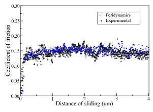
**Figure 3.** Peridynamics and experimental results [Lu and Komvopoulos 2001] of the coefficient of friction of an *a*-C film versus sliding distance for  $P = 400 \,\mu\text{N}$ .
