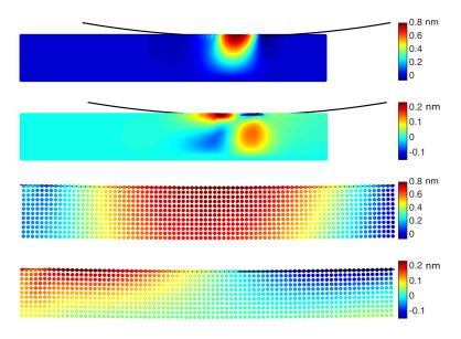
**Figure 5.** Contour maps of y-displacement (top image) and x-displacement (second image) of particles in film #4 for x/S = 1, and corresponding high-magnification contour maps (bottom two images) showing the displacement of particles in the near-surface region of the film adjacent to the contact interface with the sliding rigid tip.
