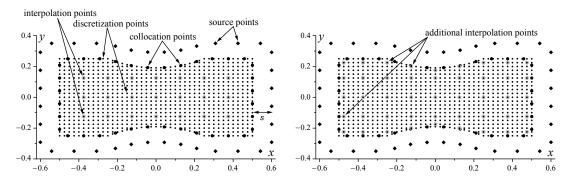
**Figure 3.** The distribution of the source, collocation, interpolation and discretization points.
