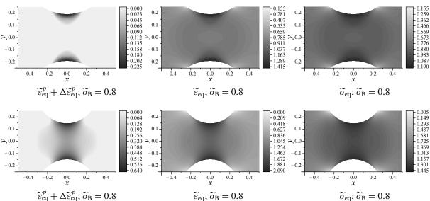
**Figure 8.** The comparison of the equivalent plastic strains  $\widetilde{\varepsilon}_{eq}^p + \Delta \widetilde{\varepsilon}_{eq}^p$  (left), the equivalent total strains  $\widetilde{\varepsilon}_{eq}$  (middle) and the equivalent stress  $\widetilde{\sigma}_{eq}$  (right) in the plate of the geometry 1-A (top) and 1-B (bottom), respectively.
