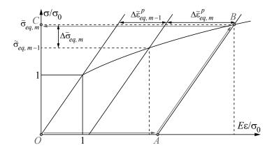
**Figure 5.** The stress-strain curve with the path *OABC* [Mendelson 1968] that allows to obtain the equivalent stress  $\widetilde{\sigma}_{eq}$  from the equivalent plastic strain increment  $\Delta \widetilde{\varepsilon}_{eq}^p$ .
