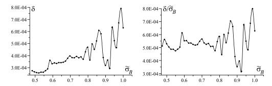
**Figure 7.** The root mean square error (left) and the root mean square error normalized with  $\tilde{\sigma}_B$  (right) of the boundary conditions fulfillment obtained for the plate of the geometry 1-B after a constant number of eight iteration steps.
