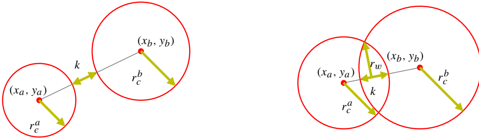
Figure 7. Two situations of two circles: (left) disjoint circles and (right) circles intersecting at two points.
