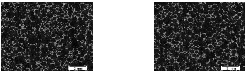
Figure 2. Images of cross-sections of the alumina foam with porosity of 86% obtained using computer microtomography: cross-section of the foam at the level \frac{1}{4} of its height (left), cross-section of the foam at the level \frac{1}{2} of its height (right) [Nowak 2014].
