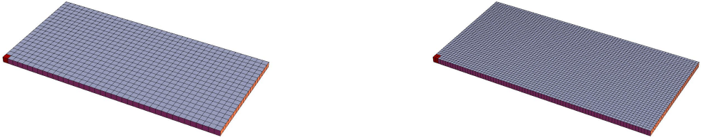
Figure 1. Finite element discretizations of plate in tension: mesh 1 (left) and mesh 2 (right); imperfection marked with red color.
