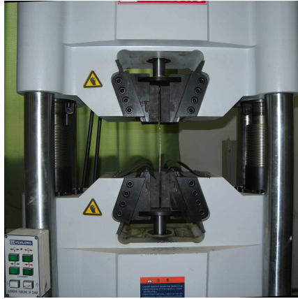
Tensile test of steel specimen
