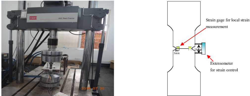
Figure 2. Testing rigs and the locations of the strain gage and extensometer for strain measurements.
