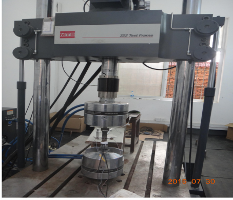
Figure 2. Testing rigs and the locations of the strain gage and extensometer for strain measurements.
