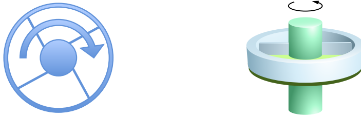
Figure 4. Torsional snap through element with negative incremental torsional rigidity. Left, top view; right, perspective view.
