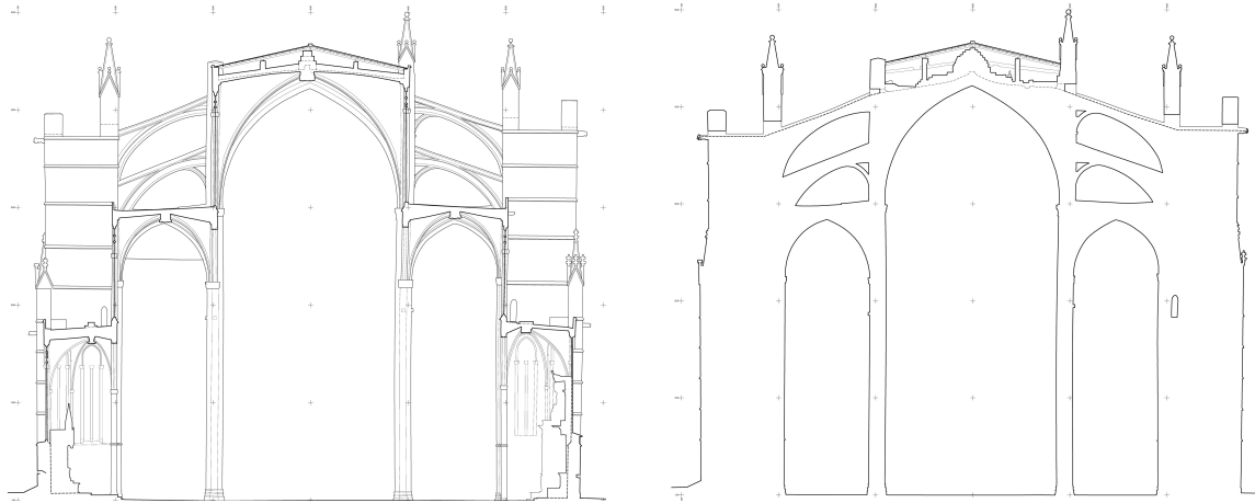
Figure 7. Cross-section of the cathedral of Mallorca: through the center of the fifth bay (left) and through the fifth pillars (right) [Fuentes and Guerra 2015].
