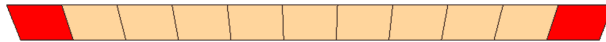
Figure 5. Vertical cut on the typical flat arch bonded according to the \frac{1}{3} rule.
