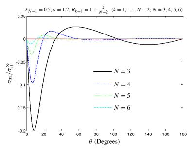
**Figure 5.** The stress disturbance  $\sigma_{32}/\sigma_{31}^{\infty}$  along the coating/matrix interface |z| = 1 on the matrix side for N = 3, 4, 5, 6 when the matrix is subjected to  $\sigma_{31} \neq 0$ ,  $\sigma_{32}^{\infty} = 0$ .
