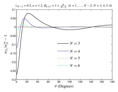
**Figure 6.** The stress disturbance  $\sigma_{31}/\sigma_{31}^{\infty} - 1$  along the coating/matrix interface |z| = 1 on the matrix side for N = 3, 4, 5, 6 when the matrix is subjected to  $\sigma_{31}^{\infty} \neq 0, \sigma_{32}^{\infty} = 0$ .
