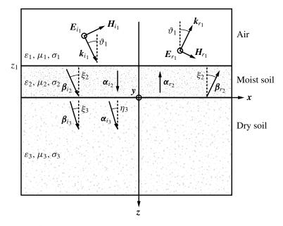
**Figure 3.** Geometry used to validate the model.
