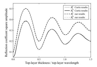
**Figure 5.** Square amplitude of the reflection coefficient for the electric field as a function of the ratio between the top-layer thickness and the top-layer wavelength in both polarizations with an incident angle of 30 degrees.
