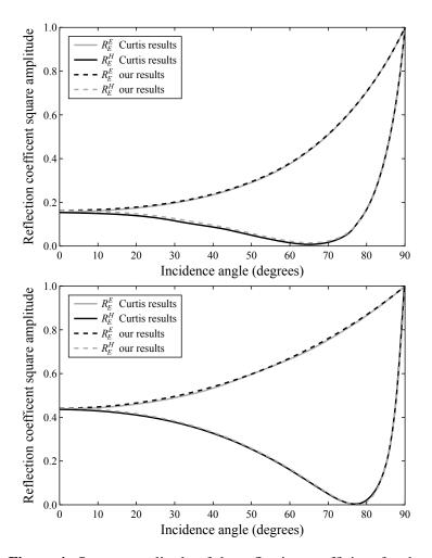
**Figure 4.** Square amplitude of the reflection coefficient for the electric field as a function of the incidence angle in both polarizations. The stratified medium is located below an air half-space and composed of a layer of moist soil 5 cm (top) and 20 cm (bottom) thick on an infinite layer of dry soil.
