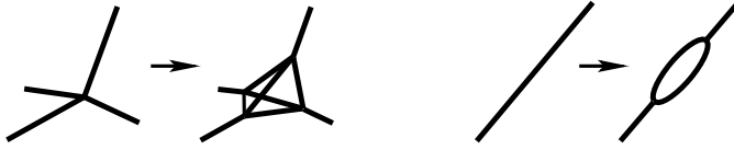
Figure 11. Some of the replacements that are needed to obtain desired unimode, bimode, trimode, or quadramode materials.
