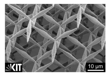
**Figure 1.** An electron micrograph of the pentamode structure created by Kadic, Bückmann, Stenger, Thiel and Wegener [Kadic et al. 2012] using a 3-dimensional lithography technique. (Used with the kind permission of Martin Wegener.)
