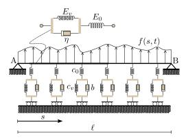
Figure 2. Planar viscoelastic beam on viscoelastic soil.
