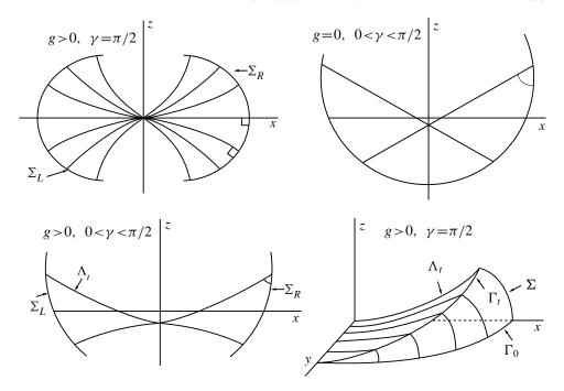
**Figure 4.** Qualitative appearance of a few exotic containers, showing the relationship of liquid surface and wall. Top row and bottom left: planar case; bottom right: three-dimensional case.
