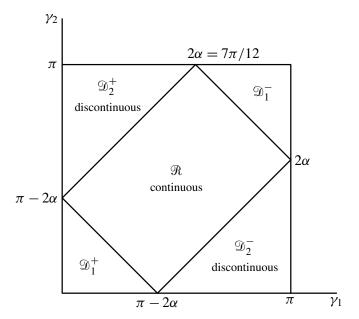
**Figure 2.** The Concus–Finn rectangle: regions in parameter space corresponding to different behaviors at a convex corner of angle  $2\alpha$ . In regions  $\mathfrak{D}_1^{\pm}$  there is no bounded graph.
