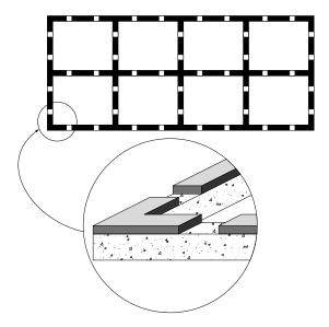
Figure 2. System of strip isolators in wall building.
