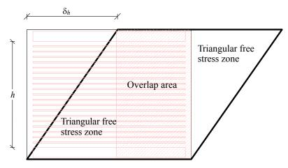
**Figure 1.** Overlap area between the top and bottom of the bearing.
