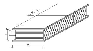
**Figure 4.** An infinite strip pad of width 2b.
