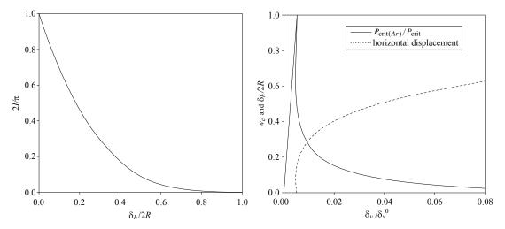
**Figure 11.** Left: moment of inertia of the overlap area against normalized horizontal displacement. Right: behavior of the bearing with real overlap area.
