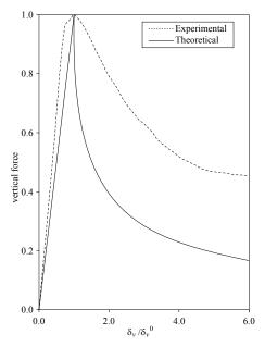
**Figure 6.** Normalized vertical force versus normalized vertical displacement from numerical experiment and analytical model.
