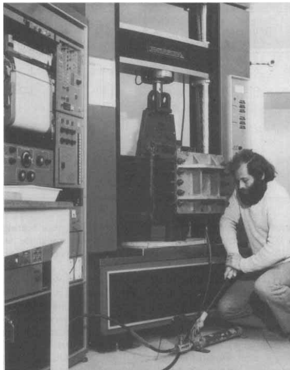
Figure 2. Lead-rubber bearing in 250 kN Instron.
