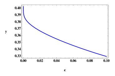
Figure 4. Reduction of normalized modulus, y, for an annular pad.
