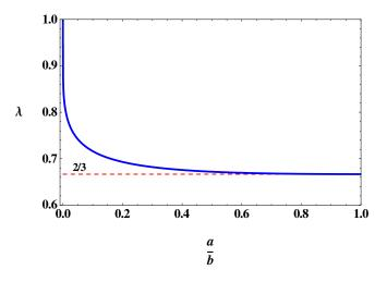
Figure 3. Reduction of compression modulus,  $E_c$ , for an annular pad [Kelly 1997].
