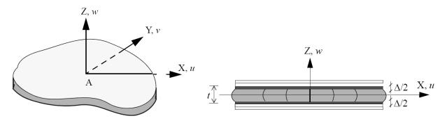
Figure 1. Constrained rubber pad and coordinate system.
