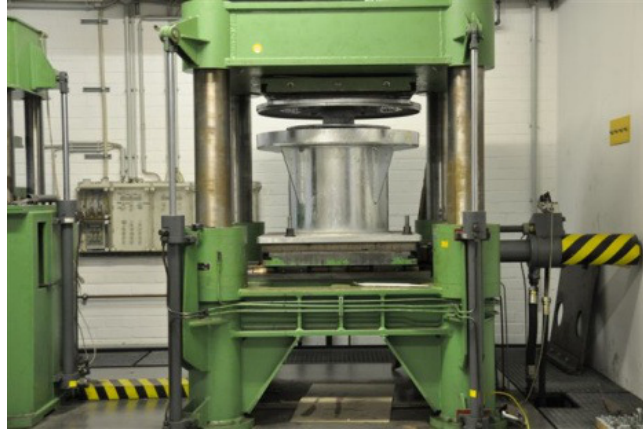
Figure 27. Viscodamper® in test rig.
