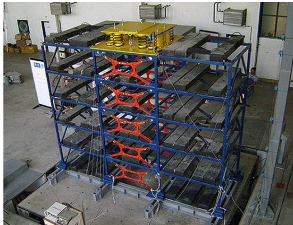
Figure 2. Shaking table test of TMCS.
